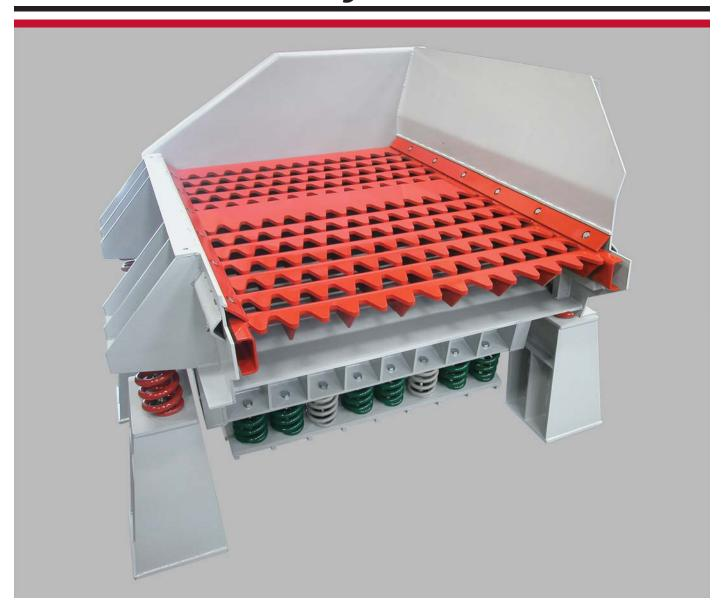
This Kraus Series 923 EZ-WERK™ Vibratory Shakeout is a natural frequency vibratory shakeout which handles up to 60 inch square by 30 inch high molds, weighing up to 10,000 pounds, at a rate of one every fifteen minutes. It uses the proven AR hardened finger deck for longer life. The molds are dumped from a mold dump onto the side of the shakeout to meet
