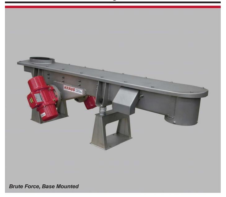
The KRAUS STEDI-FLO™ Screen Feeder is a screen and feeder combination using either a single, double or triple deck screen and a brute force drive with two electric vibrating motors. It is ideal for screening dry granular material from one inch down to 30 mesh particle size. The STEDI-FLO Screen Feeder can be
