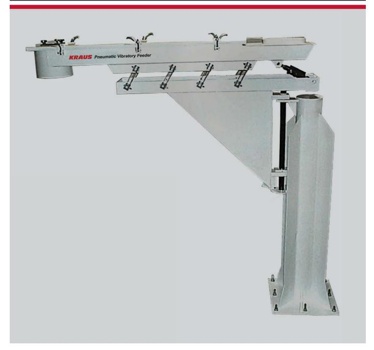
This Kraus STEDI-FLEX<sup>™</sup> Vibratory Feeder is powered by a vibrating linear air motor and is used to convey foundry sand to two (2) different core sand mixers from a single surge hopper which is fed by a dense phase pneumatic conveying system.
