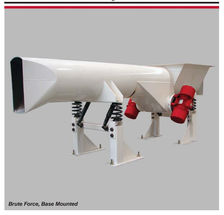
This Kraus STEDI-FLO™ Vibratory Feeder is designed to feed foundry sand to an existing bucket elevator from a surge hopper. It also includes a
