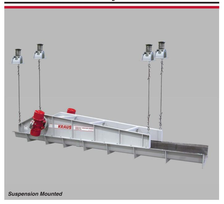
This Kraus STEDI-FLO™ Vibratory Feeder with a suspension mounting system is used for conveying sand and castings from one existing vibratory conveyor to another existing conveyor for a Midwestern foundry.
