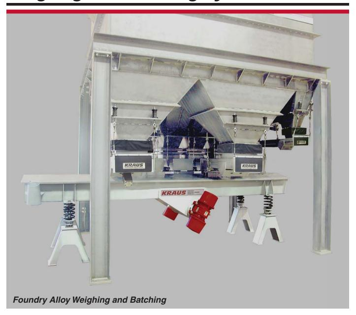
This Weighing and Batching System uses multiple L-Type Vibratory Feeders to feed individual ingredients onto one STEDI-FLO™ Vibratory Feeder. The STEDI-FLO Vibratory Feeder is mounted on four load cells, one under each spring support leg. Individual ingredients are weighed in succession until the weighed batch is complete. All L-Type
