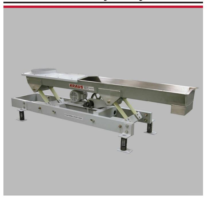
The Kraus STEDI-FLEX™ Vibratory Conveyor is low in cost and simple in design and construction, and includes a counterbalanced base specially designed to isolate the counteracting forces produced in a
