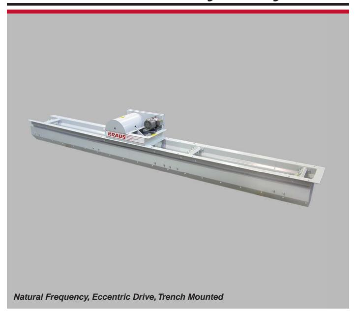
This Kraus TRENCH-TITE™ Vibratory Conveyor is set into a narrow trench, level with the floor. It is installed in an iron foundry and is used to convey spill sand during a molding operation. Special features include a flexible polymer conveying trough which flexes and prevents any sticky foundry molding sand from adhering
