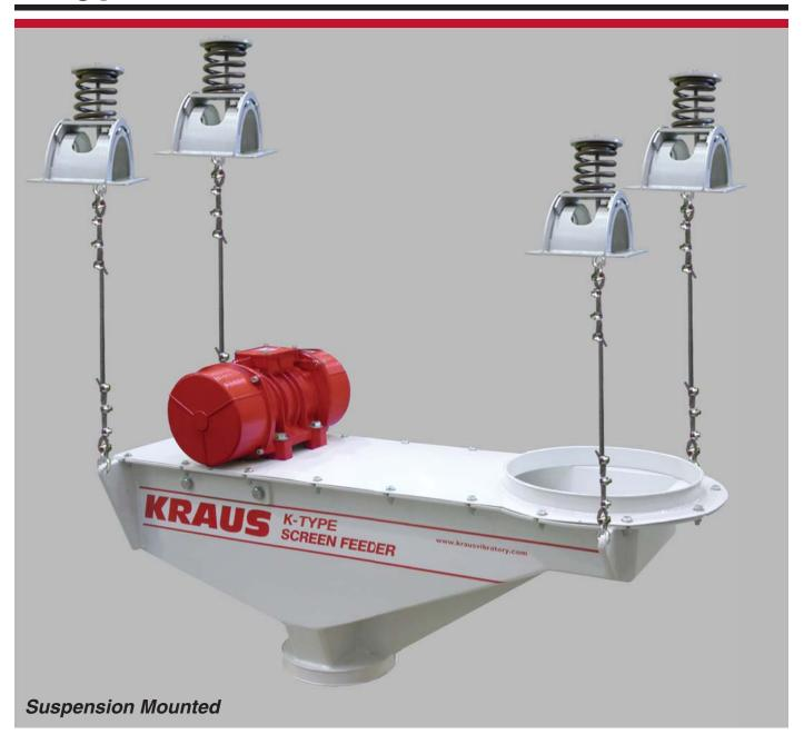
The Kraus K-Type Screen Feeder is a screen and feeder combination using a single or double deck screen with a brute force drive and a single electric vibrating motor. It is ideal for screening dry granular material from one inch down to 100 Mesh particle size. The K-Type Screen Feeder can be flood fed and mounted directly below any size surge hopper
