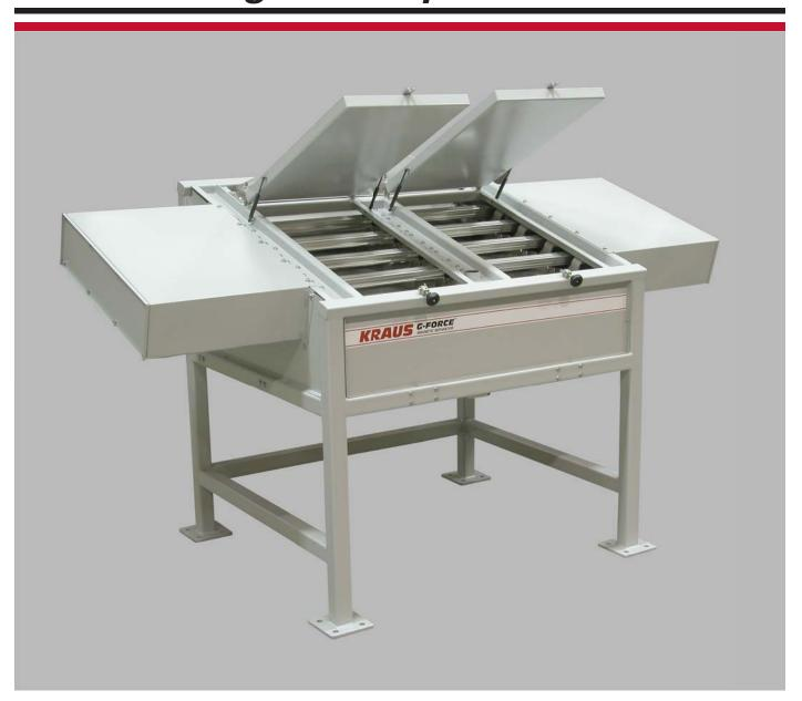
The G-Force<sup>™</sup> Magnetic Separator by Kraus Vibratory Equipment was designed for magnetically separating fugitive metal particles from almost any dry bulk granular product, such as the removal of plastic pellets which may contain metallic particles. This particular model has the ability to operate continuously and contains multiple magnetic rods with automatic wipers to continually keep them clean of magnetic particles. The product flows
